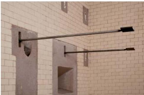
128 measuring points record the temperatures of the samples and 28 measuring points the temperature in the furnace
