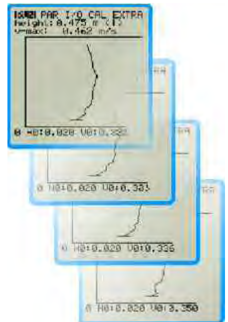
Direct flow profile indication on the display
