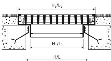
$$\begin{aligned} H_1 &= H-20 & H_3 &= H+32 \\ L_1 &= L-20 & L_3 &= L+32 \end{aligned}$$
