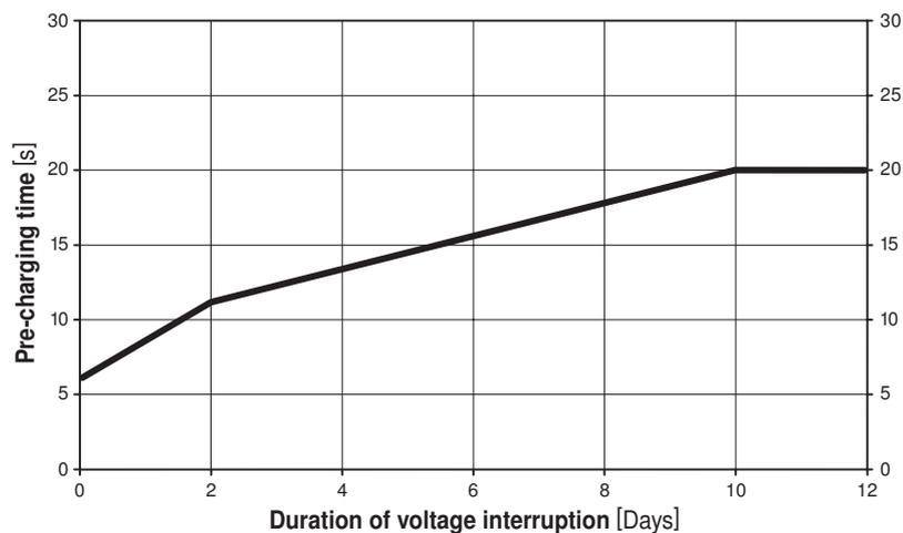
**Delivery condition (capacitors)** The actuator is completely discharged after delivery from the factory, which is why the actuator requires approximately 20 s pre-charging time before initial commissioning in order to bring the capacitors up to the required voltage level.
