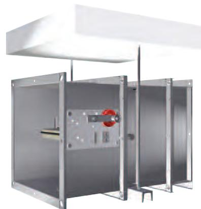
The fire dampers are suspended using threaded rods. The rods can be bare if their length does not exceed 1.50 m; longer rods require insulation.
