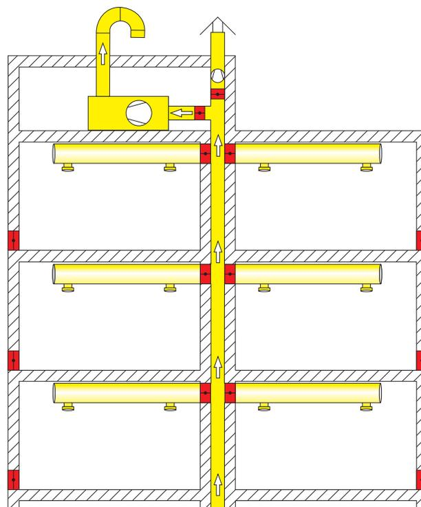
Ventilation with a combined ventilation/smoke extract system
