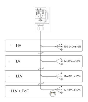
If the PoE energy version, to guarantee the isolation required by IEEE for ethernet, the external power supply must be protected at least 1500Vac with respect to a ground and any other connection.
