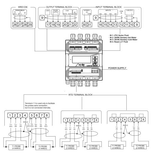
Cable gland PG7: Allowed diameter cables 3-6.5 mm.
