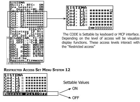
**Restrict = ON:** Access permitted only to functions provided for a specific level; Exemple: If the operator has a code of access level 3, after having set it, he will can change only the functions provided for a access level 3.
