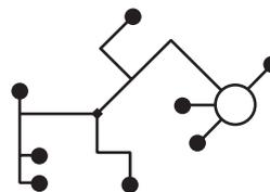
There are no restrictions for the network topology (star, ring, tree or mixed forms are permitted). Supply and communication in the same 3-wire cable
