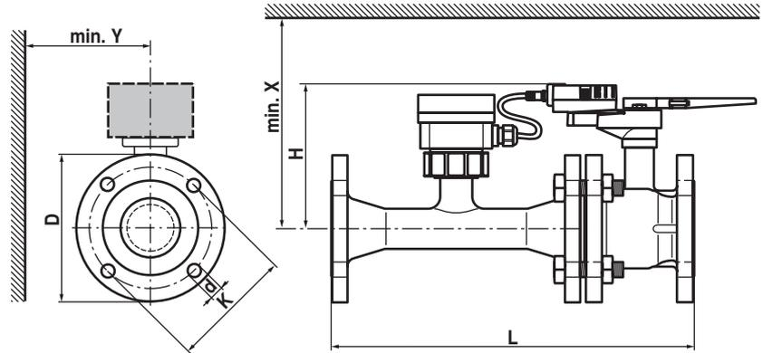
If Y < 180 mm, then the extension of the hand crank must be dismantled as necessary.
