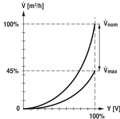
**Creep flow suppression** Given the very low flow speed in the opening point, this can no longer be measured by the sensor within the required tolerance. This range is overridden electronically.
