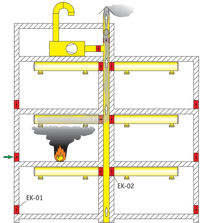
Smoke extract operation of a combined ventilation/smoke extract system
