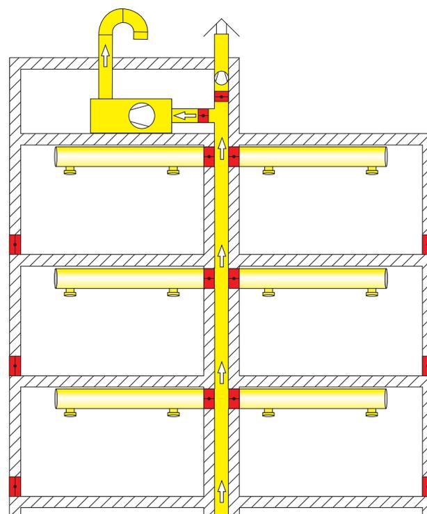
Ventilation with a combined ventilation/smoke extract system
