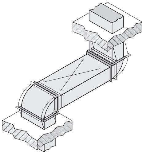
The LüAR requirements for force and load protection apply also to the installation of fire dampers. These must be connected by means of combustible flexible connectors made of normal flammable building materials (material classification B2 in compliance with DIN 4102) and these
