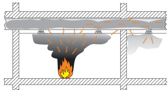
Spread of fire and smoke through ventilation ducting
