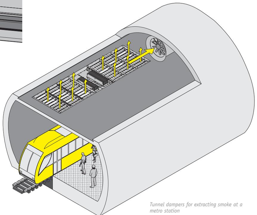
Tunnel dampers for extracting smoke at a metro station
