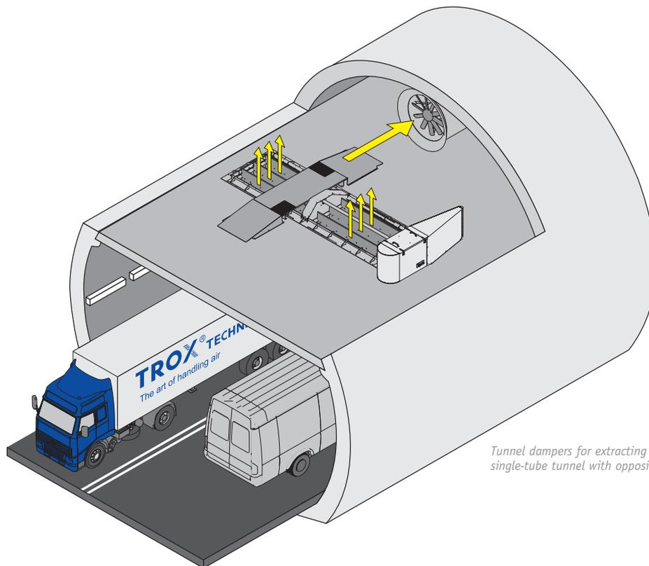
*Tunnel dampers for extracting smoke from a single-tube tunnel with opposing traffic flow*
