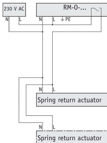
Diagram shows “power off”, i.e. fire damper or smoke control damper closed
