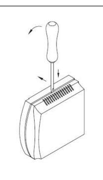
To open the enclosure, set a screwdriver (2.0) in the groove at centre, press down, and lift up the bottom frame slightly. Pull top cover forward and hold it.
